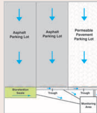
Permeable Pavement Parking Lot
